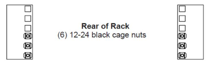
Step 2. The rail kit is pre-set for rack depths of 25.75" to 31.5" [654mm to 800mm]: If your rack is less than 25.75" [654mm] deep, move the hardware attaching the Rear Slider brackets to get the needed adjustment range. Moving the hardware attaching the Rear Slider can achieve any depth from 13" to 31.5" [330mm to 800mm]. The Angle Bracket(s) may need to be removed.
