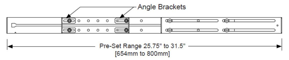
"Right" Rail in the new 2Post Flush Configuration
