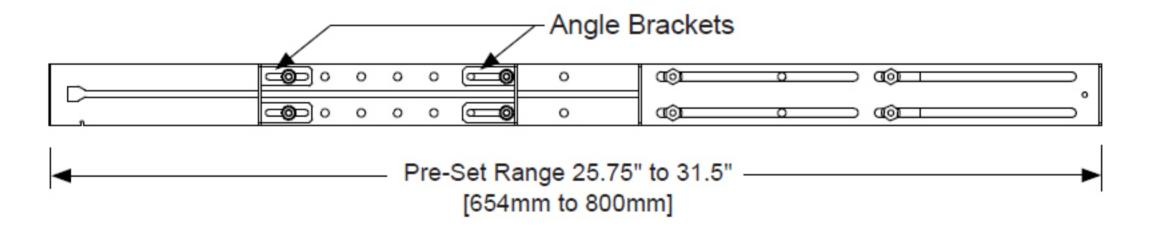
Step 3. Attach the front and rear of both rails to the rack using supplied screws at each rail end: Tighten the front and rear Pan Head Screws on the right side rail.
