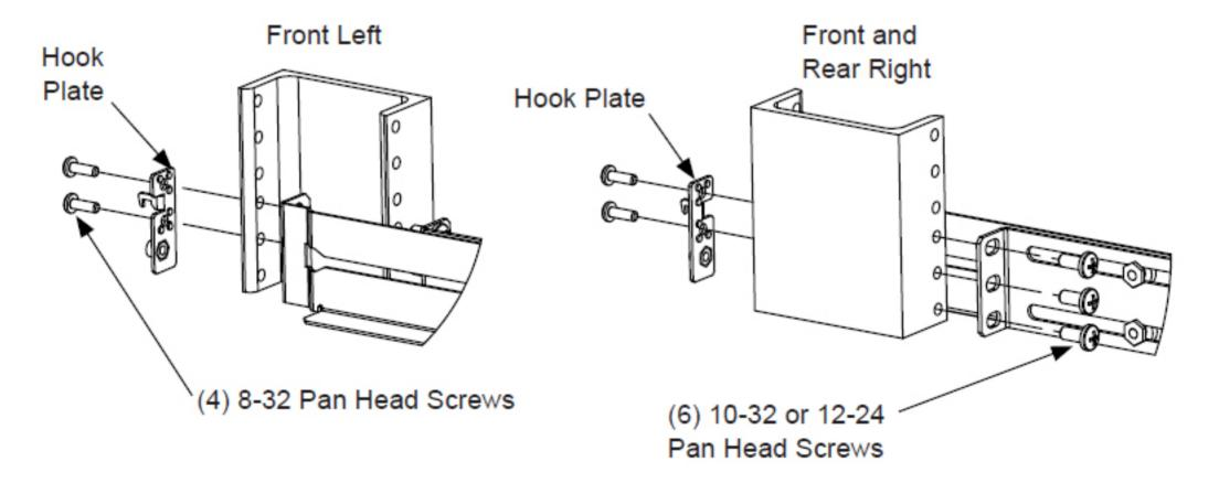
**Note:** When tightening the loose rails, support the bottom of the server to ensure proper rail adjustment.
